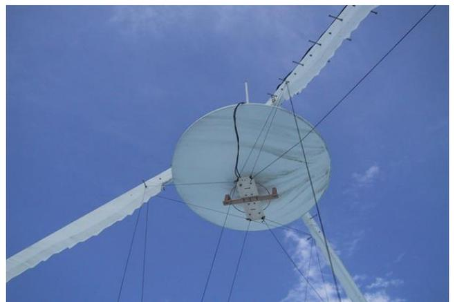
Fig. 15 “Marionette style” tension cable mechanism
